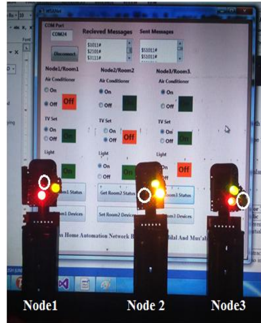
Figure 13: System Nodes after settings And the Software, the white circle highlights the Off LED
